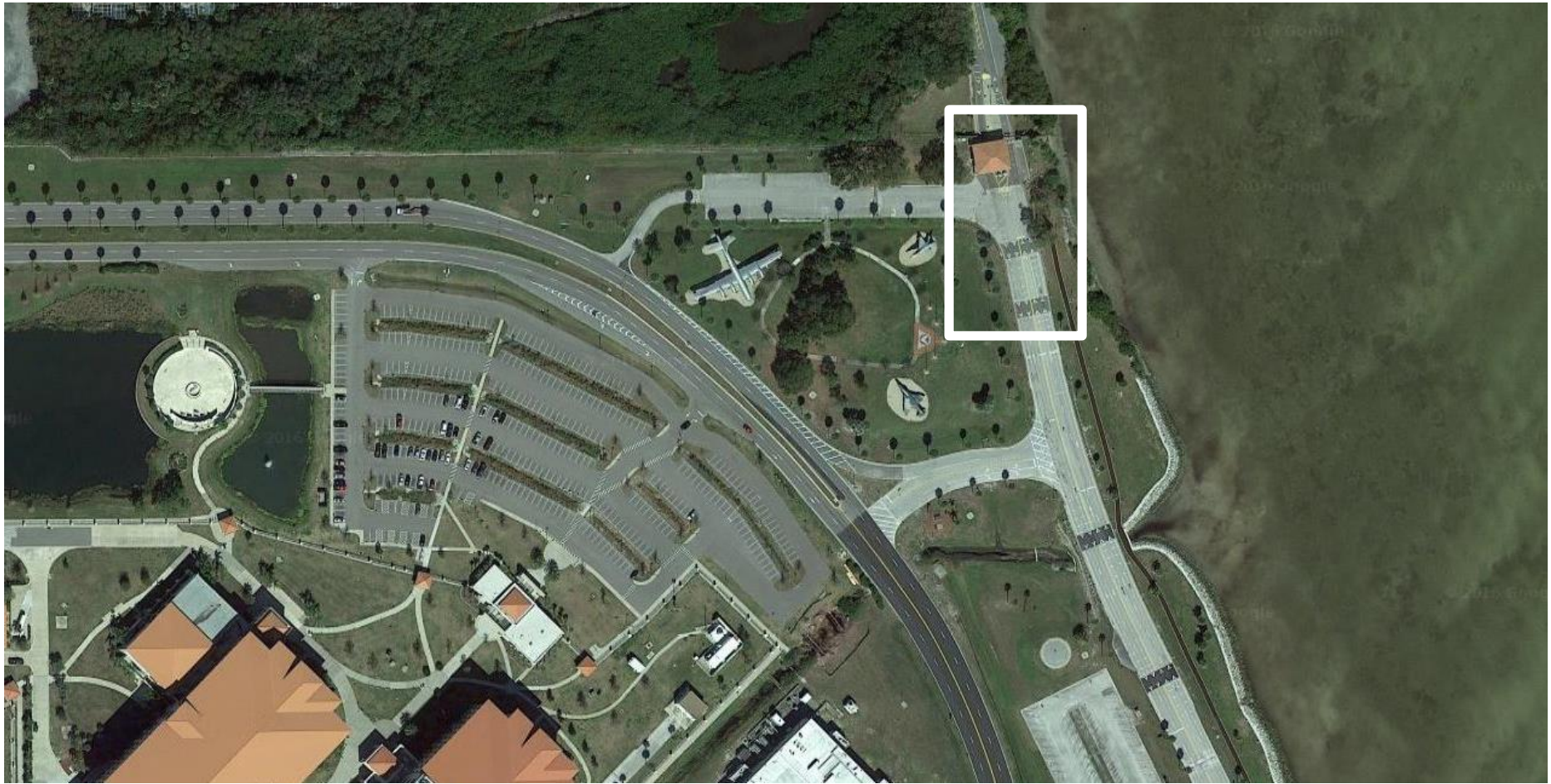
Figure 1 – Aerial view showing the general areas of work for the proposed Bayshore Gate improvements. The project adds an overhead canopy over inspection areas and an additional 3,000 sf of pavement to facilitate turning vehicles around. A wider view of this area is shown in Figure 2.
